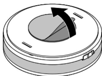
2. Remove the protective film from the back of the adhesive pad.
